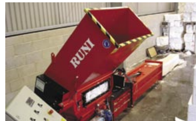
Details of some machines suitable for cold compaction or thermal densification
